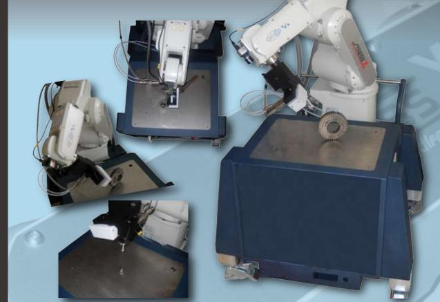
Stress-X allows to measure residual stress, providing a through non-destructive analysis of samples of any dimensions tank to the original mounting of the diffractometer head on a 6 anthropomorphic axis robot.
